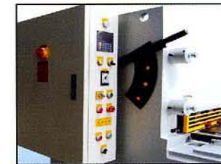
CENTRALIZED CONTROL PANEL
